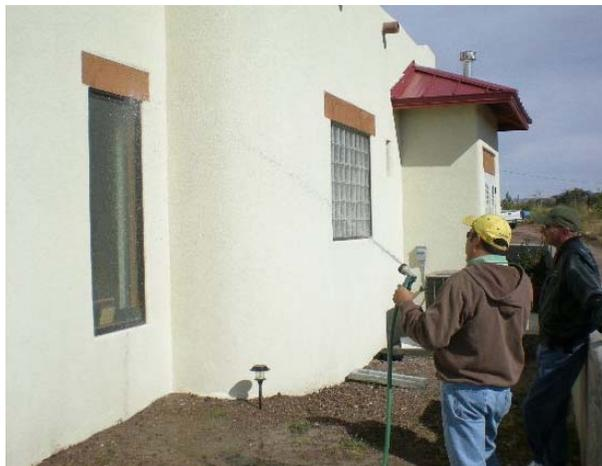
Figure 7 – Non-calibrated hose test being performed.
