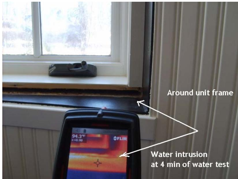
Figure 9 – Infrared imager documents water intrusion.
