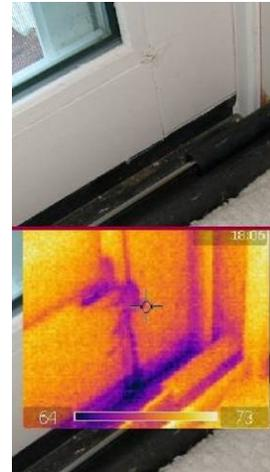
Figure 3b – Water intrusion at a door.
