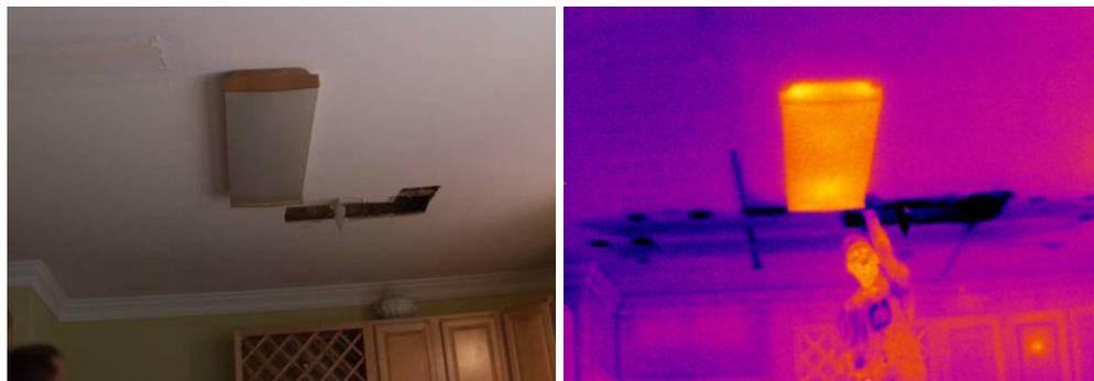
Figure 4 – Plumbing fixture leak in a house, found in seconds with an infrared imager.
