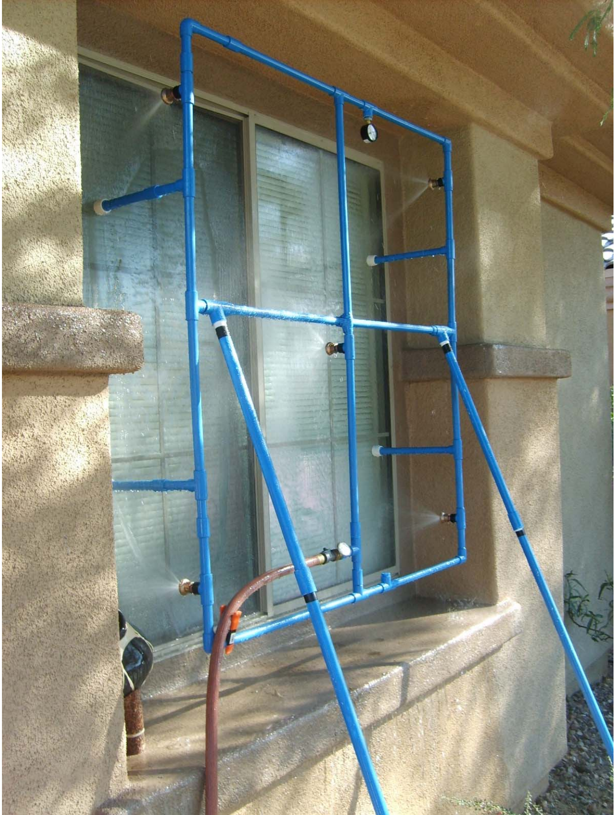
Figure 9 – Calibrated spray rack set-up.
